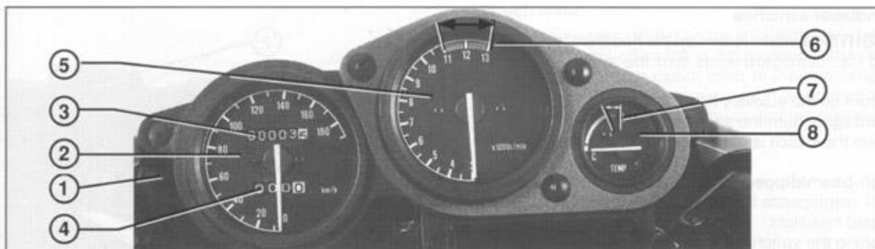
1. Trip counter reset - 2. Speedometer - 3. Odometer - 4. Trip counter - 5. Rev counter - 6. Rev counter red area - 7. Engine temperature gauge red area - 8. Engine temperature gauge
